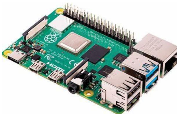
**Fig. 1.** Placa Raspberry Pi 4B
